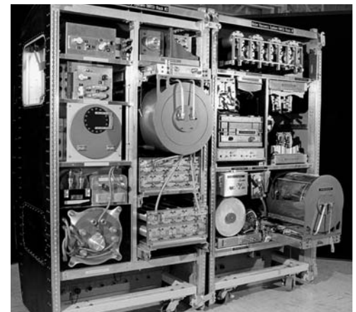
This is a close-up view of the Environmental Control and Life Support System (ECLSS) Water Recovery System (WRS) racks. The WRS provides clean water through the reclamation of wastewaters, including water obtained from the Space Shuttle's fuel cells, crewmember urine, used hand wash and oral hygiene water, cabin humidity condensate, and Extravehicular Activity (EVA) wastes. The Water Recovery System (WRS) is comprised of a Urine Processor Assembly (UPA) and a Water Processor Assembly (WPA). The UPA accepts and processes pretreated crewmember urine to allow it to be processed along with other wastewaters in the WPA, which removes free gas, organic, and nonorganic constituents before the water goes through a series of multifiltration beds for further purification. Product water quality is monitored primarily through conductivity measurements. Unacceptable water is sent back through the WPA for reprocessing. Clean water is sent to a storage tank. The water must meet stringent purity standards before consumption by the crew.
